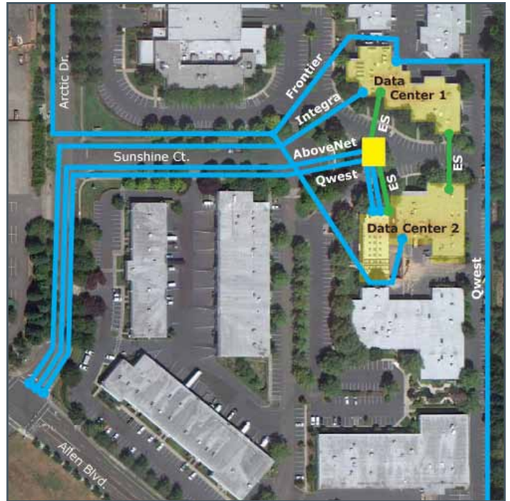
EasyStreet uses a variety of network providers, each with diverse entrances into Data Center 1 and/or Data Center 2.
